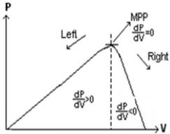
Fig-6 shows that the slope of the P-V array power curve is zero at The MPP, increasing on the left of the MPP and decreasing on the Right hand side of the MPP. The basic equations of this method are as follows.
